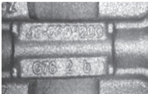
Figure A : Casting piece shotblasted with standard S-660 product
