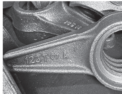
Figure B : Casting part shotblasted with our KOTAR 47 product
